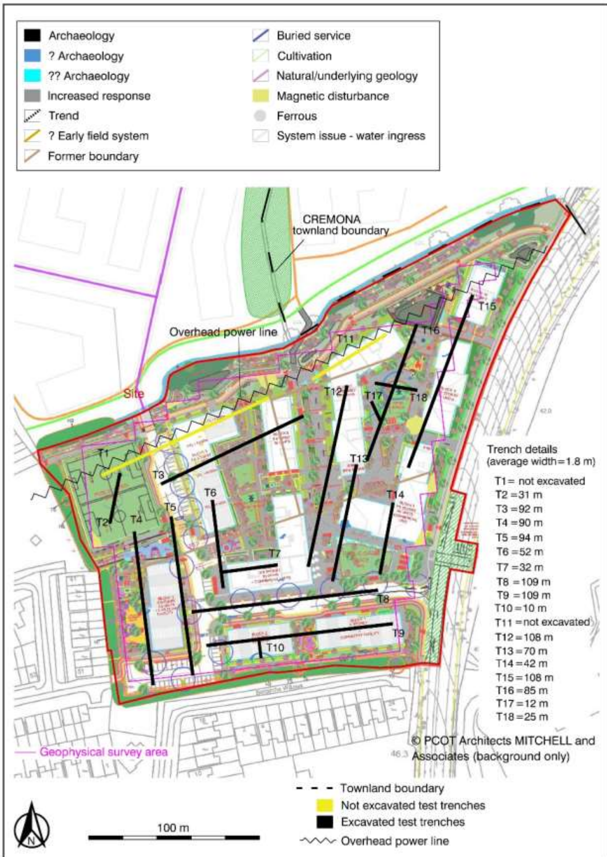
Figure 4.3 Details of proposed development showing interpretation of geophysical survey (19R0011) and excavated test trenches (19E0034).
